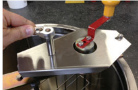
STEP 1. REMOVE BOTH BELT GUARD NUTS WITH 7/16 WRENCH
