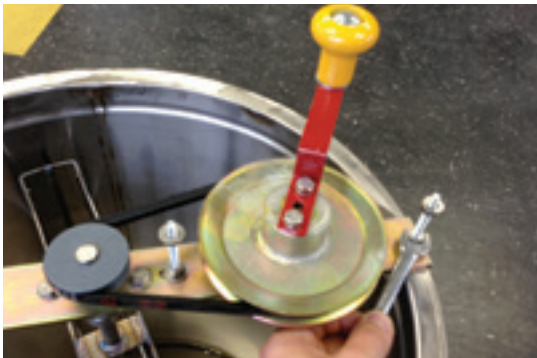
STEP 2. REMOVE BOTH BELT GUARD BOLTS
