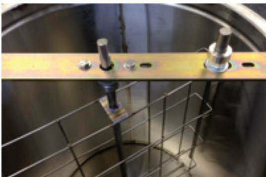
STEP 4. NOW YOU CAN LIFT BOTH PULLEYS STRAIGHT UP AND OFF THE SHAFTS
