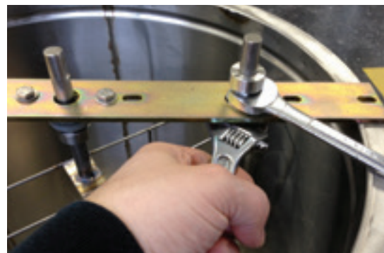
STEP 5. REMOVE HAND PULLEY SHAFT/BOLT USING A 3/4 WRENCH OR CRESCENT WRENCH. THERE IS A BOLT UNDER THE COLLAR, AND UNDER THE TOP BAR
