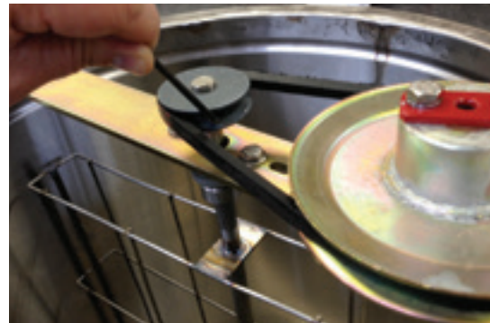
STEP 3. USE 1/8 ALLEN WRENCH TO LOOSEN SET SCREW IN PULLEY ON BASKET SHAFT
